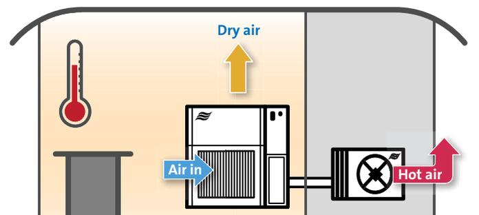
Room temperature is at or above set point. Dehumidifier dries the room without heating. Heat is expelled outside.
