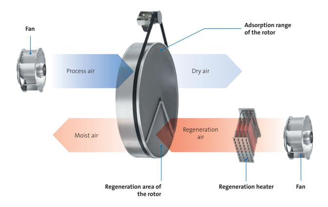
Desiccant drying - typical principle of operation
