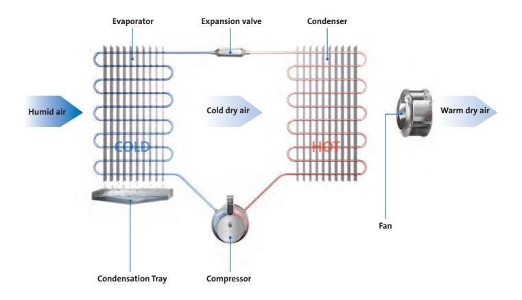
Condensing dehumidification — typical principle of operation
